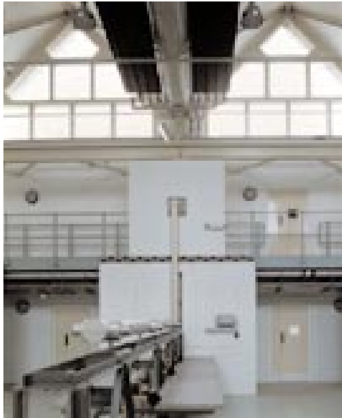
Figure 7 Gable glazing and rooflights help to achieve high light levels in the mechanical laboratories
