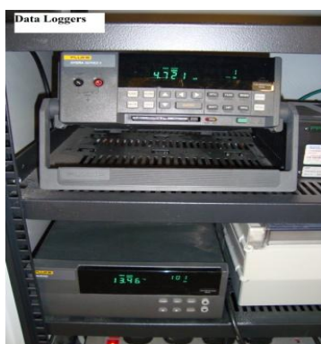
Fig.5 Data Loggers – Fluke 2640 NetDAQ and 2635 Data Bucket Data Acquisition Units
